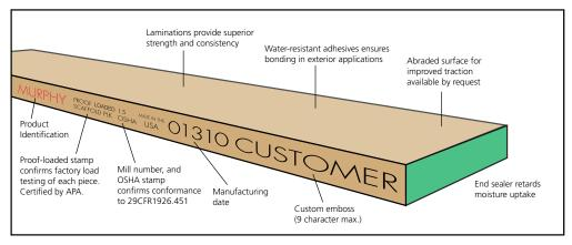
Murphy Douglas-fir Engineered LVL Scaffold Planks are machine-sawn with user-friendly eased edges and are end-sealed with Murphy Green. Each plank is embossed and inked on both edges. The stated information includes: Product Name, Scaffold Plank, APA Mill # 1089, Manufacturing Date, and OSHA 29CFR 1926.451 conformance.
